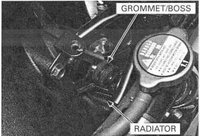
Install and tighten the radiator upper mounting bolt.
