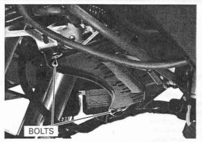
Remove the intake air duct mounting screws. Remove the intake air duct from the air cleaner housing.
