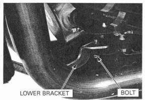
Install and tighten the radiator lower mounting bolt.
