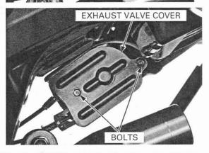
between the muffler and rear fender B.
