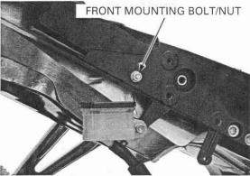
Install the muffler assembly and temporarily install the muffler rear mounting bolts.
