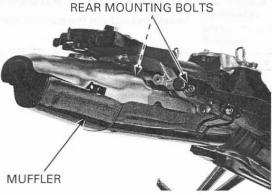
Install the muffler front mounting collar and bolt.
