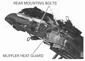
Install the muffler heat guard front mounting bolt and nut.
