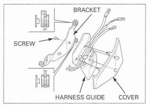
Install the right cover onto the rear fender A bracket, tighten the screw.
