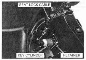
Hook the seat lock cable to the seat lock lever.
