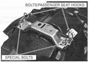
Install the passenger seat rear hook and tighten the pan screw securely.
