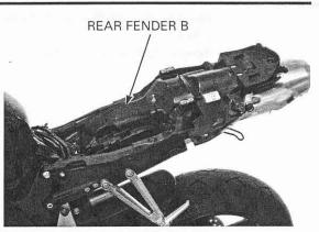
Install the rear fender B-to-heat protector trim clips and secure them.
