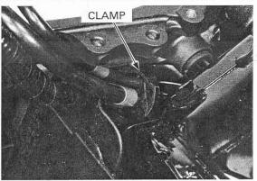
Install the rider seat bracket onto the seat rail. Install and tighten the rider seat bracket mounting bolts and nuts to the specified torque.
