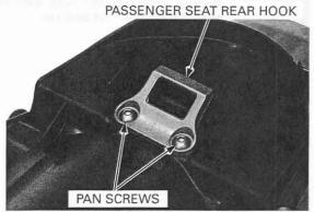
Remove the flange bolts and passenger seat hooks. Remove the passenger seat hook special bolts, then remove the passenger seat bracket.
