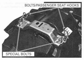
Unhook the seat lock cable from the seat lock lever, then remove the passenger seat bracket.
