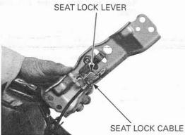
Disconnect the seat lock cable from the seat lock key cylinder.
