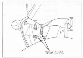
Remove the middle cowl-to-upper cowl pan screws. Remove the middle cowl-to-inner middle cowl special screws and middle cowl mounting special screw.
