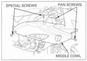
Remove the middle cowl while releasing the hooks on the upper cowl.
