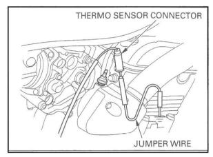
Turn the ignition switch ON and check the coolant temperature gauge.
