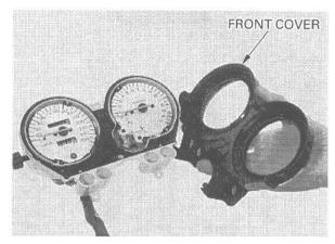
Remove the six terminal screws and tachometer/indicator unit.
