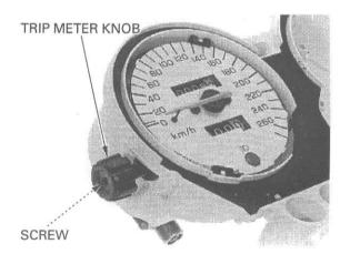
Remove the two speedometer gearbox screw, then remove the speedometer unit.
