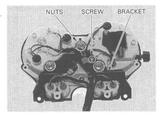
Remove the front cover mounting screw.
