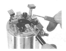
Inspect the brushes for damage and measure the brush length.
