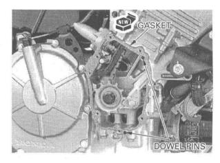
Apply sealant to the threads of the two bolts indicated by " $\triangle$ " mark on the cover.
