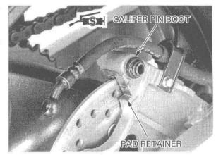
Install the pad spring into the caliper body.
