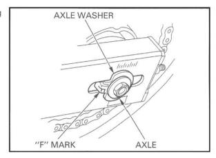
Install the axle washer with its "F" mark facing forward.
