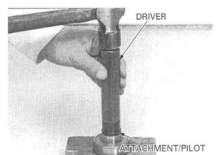
Drive the new driven flange bearing into the driven flange using the special tools.
