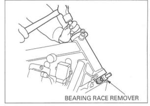
Install the steering stem nut onto the stem to prevent the threads from being damaged when removing the lower bearing inner race from the stem.
