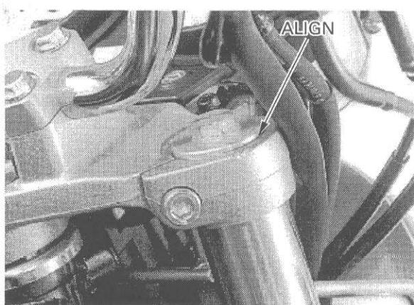
Tighten the bottom bridge pinch bolt.
