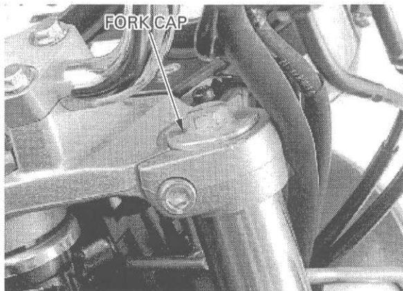
Tighten the fork top pinch bolt to the specified torque.
