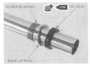
Drive the oil seal in using the special tools.
