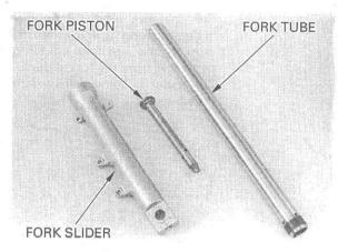
Check the fork piston ring for wear or damage. Check the rebound spring for fatigue or damage.
