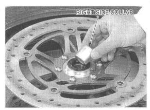
Install the front wheel between the fork legs while aligning the left brake disc between the left brake caliper pads.
