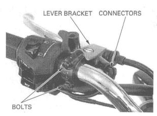
Remove the left handlebar switch screws.
