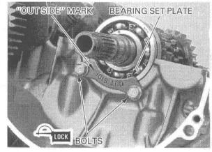
Install the dowel pin and bearing set ring on the upper crankcase.
