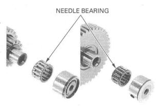
Check the gear dogs, dog holes and teeth for abnormal wear or lack of lubrication.
