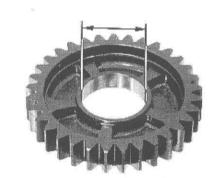
Measure the I.D. and O.D. of each gear bushing.
