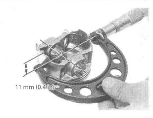
Measure the piston pin bore.
