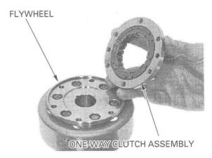
Clean and apply a locking agent to the starter clutch outer mounting bolt threads.
