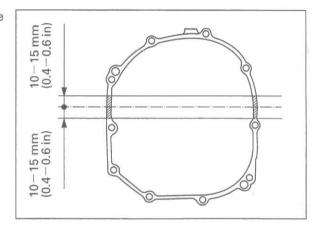
Install the dowel pins and new gasket.
