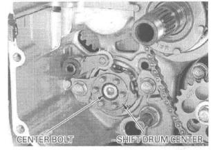
Install the thrust washer and gearshift spindle assembly into the crankcase while aligning the spring ends with the crankcase stopper pin.
