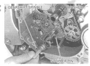
Install the gearshift pedal link aligning its slit with the punch mark on the gearshift spindle. Install and tighten the pinch bolt to the specified
