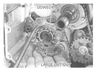
Apply a locking agent to the shift drum center socket bolt threads.
