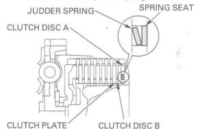
Install the pressure plate to the clutch center aligning the punch marks between the clutch center and pressure plate. 9-9
