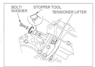
Remove the bolts, sealing washers and cam chain tensioner lifter.
