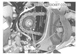
Tighten the drive sprocket cover bolts.
