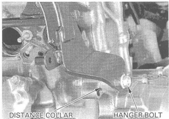
Install the front right engine hanger bracket and tighten the bolts to the specified torque.
