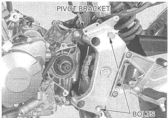
Install and tighten the swingarm pivot bolt to the specified torque.
