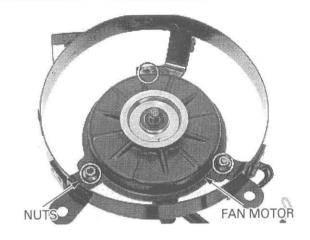
Install the cooling fan onto the fan motor shaft by aligning the flat surfaces.
