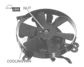
Install the fan motor/shroud assembly onto the radiator.
