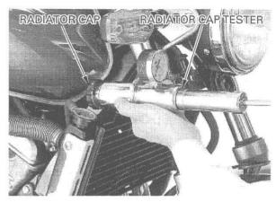
Pressure the radiator, engine and hoses, and check for leaks.
