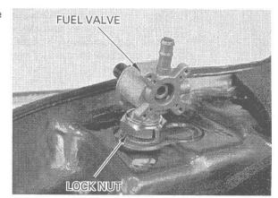
Remove the fuel strainer and O-ring from the fuel valve.
