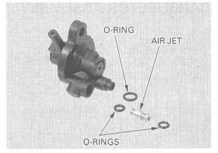
Install the air jet and air cut-off valve onto the carburetor.
