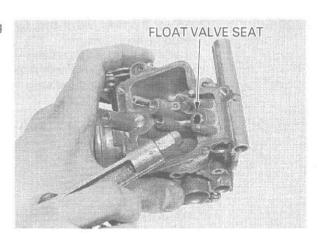
Blow open each air and fuel passages in the carburetor body with compressed air.
