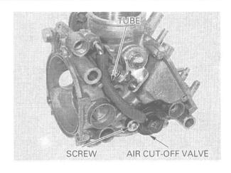
Remove the air cut-off valve, air jet and O-rings.
