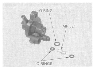
Clean the fuel strainer in the float valve seat using compressed air from the float valve seat side.
