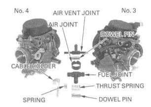
Remove the screws and throttle cable holder from the No.3 carburetor.
