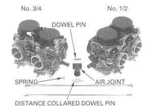
Separate the No.1 carburetor from the No.2 carburetor.
