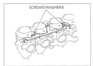
Loosen and remove the carburetor connecting 6 mm nut and 5 mm nut.
