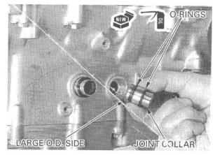
Apply oil to the new O-ring and install it into the groove of the oil cooler base.
