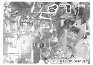
Install and tighten the oil cooler assembly mounting bolts.
