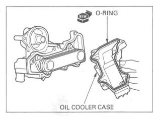
Assemble the oil cooler case and oil cooler base, then install the sealing washer and bolts. Tighten the bolts securely.
