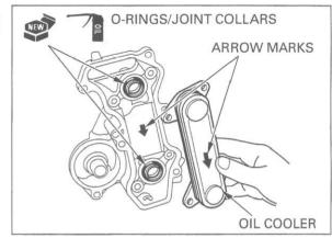
Install the washers and bolts, tighten the bolts securely.
