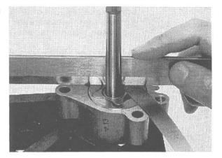
Measure the oil pump driven sprocket collar O.D.
