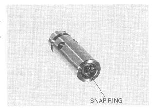
Inspect the piston for wear, sticking or damage. Inspect the spring for weakness or damage.
