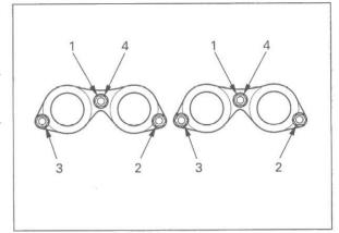
Install the exhaust pipe mounting bolt/nut and tighten the nut to the specified torque.
