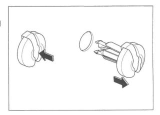
Raise the center pin by pushing the retaining tabs back.
