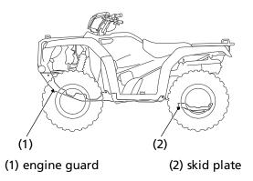
The engine guard (1) protects the frame, front final gear case and engine crankcase.
