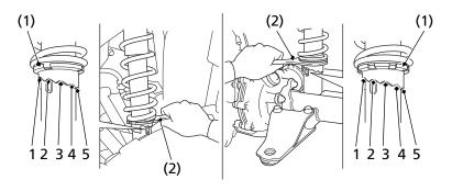
(1) spring pre-load adjuster(2) pin spanner
