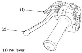
(2) rear brake lever/parking brake lever
